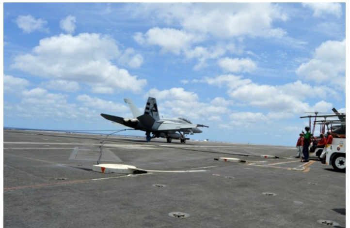
VX-23 F/A18-F Super Hornet catches the arresting gear wire while landing aboard USS George Washington while testing the MAGIC CARPET carrier landing assistance technology.
