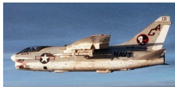
The AGM-45A was used in combat by many different types of tactical aircraft in South East Asia, including the A-4, A-6, A-7, F-4, and F-105G. It was controlled in flight by its forward cruciform wings. It could use three different blast-fragmentation warheads, the 67.5 kg (149 lb) MK 5 MOD 0 and MK 86 MOD 0, and the 66.6 kg (147 lb) WAU-8/B, and employed a dual-mode (proximity and impact) fuse.
